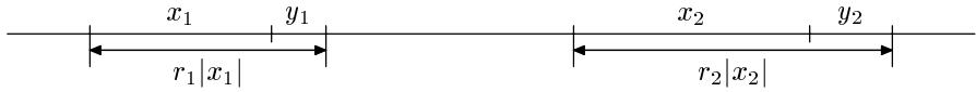
Fig. 1. Two fractional powers of exponent r_1 and r_2 are implanted; y_i is a prefix of x_i (in this example the exponents are less than 2, so only one full period is shown)
